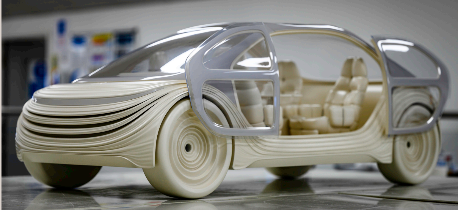
As part of a recent commission by IM Motors, Ogle produced a 1200mm-long model of a visionary all-electric concept car for Heatherwick Studios, created entirely with Stratasys' SL technology.
